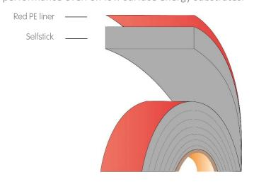
Thickness: 1,6 mm (0.062 inch)  $\pm$ 10% Core: Closed cell acrylic Adhesive: Closed cell acrylic Density: 880 kg/m³ (54lb/ft³)
